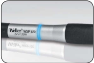
visual process control via blue LED light ring Selectable stand-by mode with visual process control via blue LED light ring on most models (light on = heater on, light is blinking = Standby or heating up light off = heater off)
