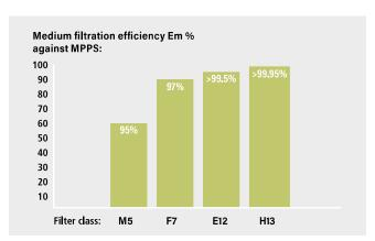
Filter Class M5, F7: Fine dust filter as per EN 779:2012
