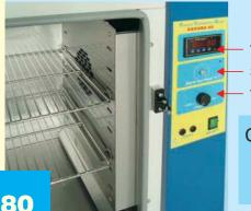
Temperature Control Safety thermostat Ventilation opening
