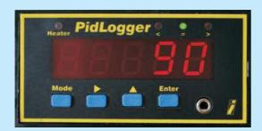
Temperature electronic control with PID regulator and multifunction timer.
